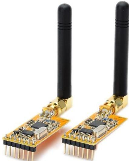
Figura 3: Radiotransmissor APC-220.
